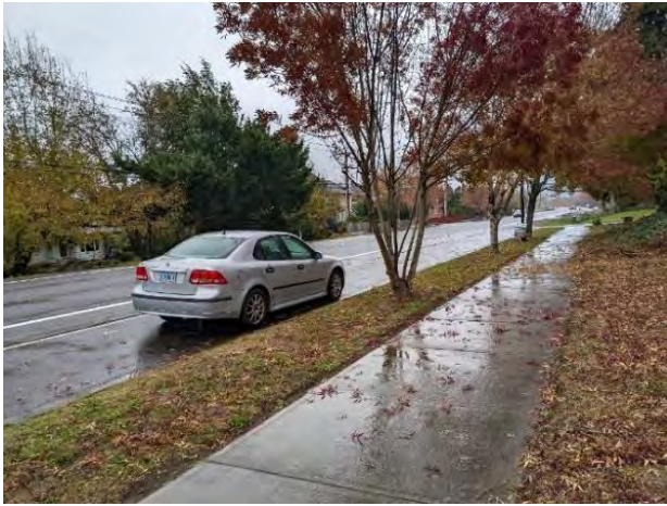
Image 3: Sidewalk Buffered by a Planting Strip and Parking Lane in Troutdale (Residential Context)
