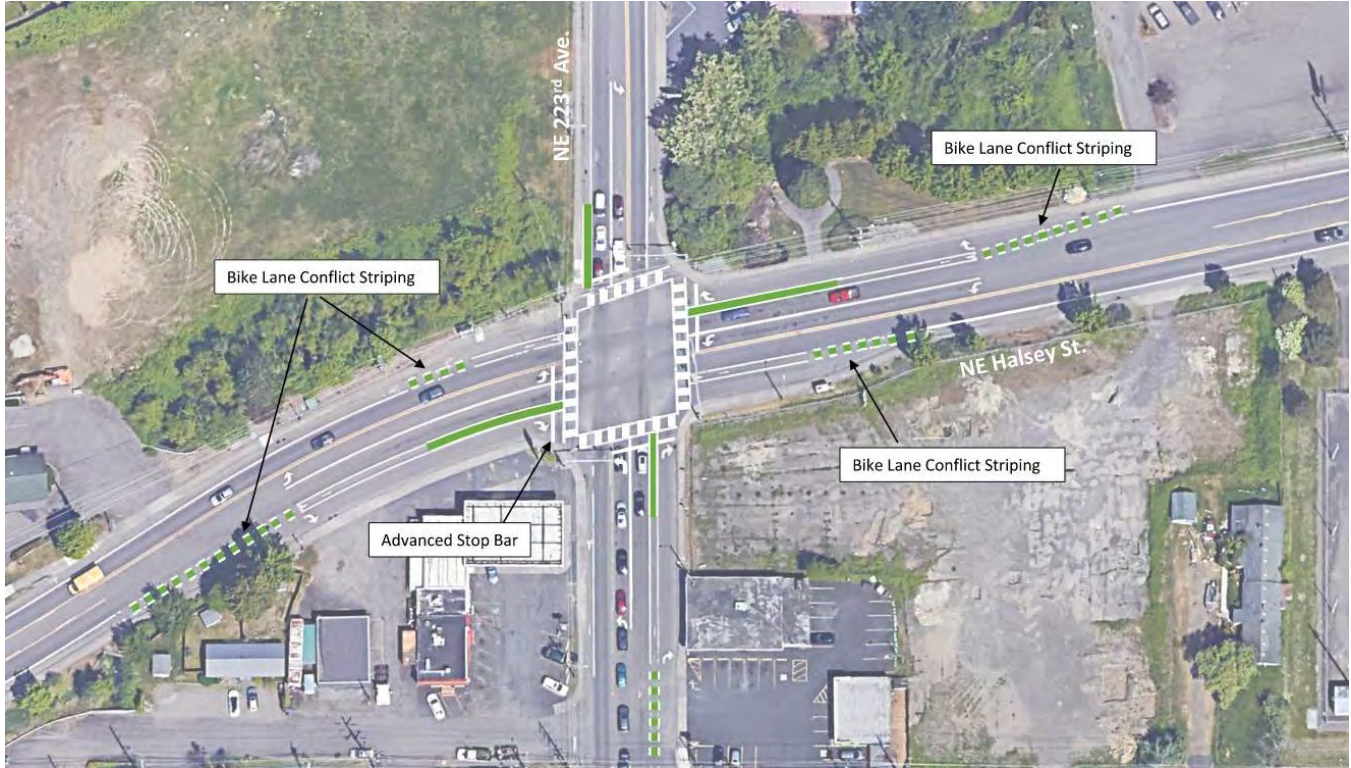
Figure 5. Near-term Intersection Treatments – NE 223 rd Avenue
